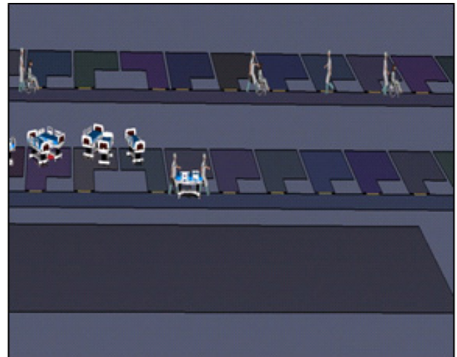
Picture 4. Simulation moment for the second scenario when no elevator is working and when the main and auxiliary stairs are available
